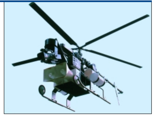
Power Sonix AeroVoice PA system on board an unmanned airborne vehicle.
